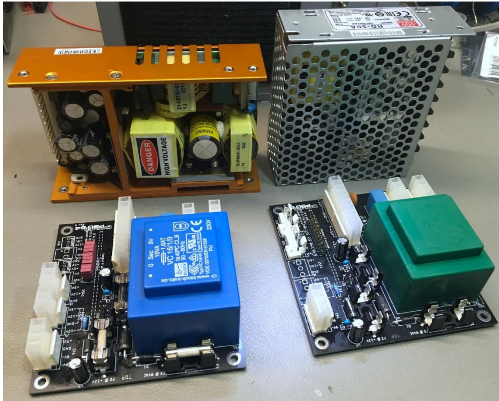
Figure 26: two versions of the PSU Combi
