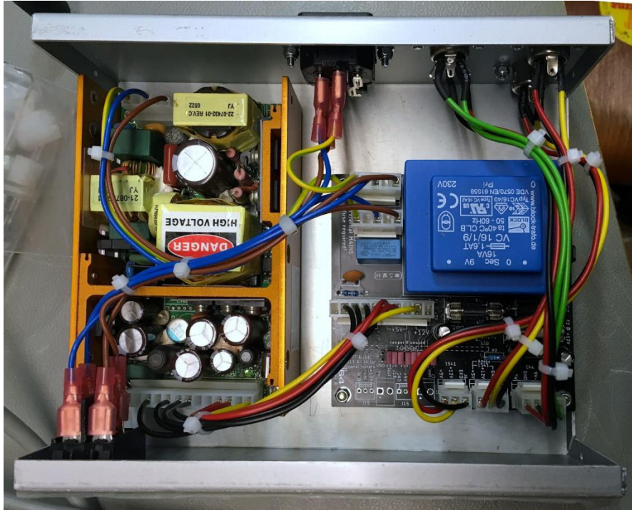
Figure 27: Finished PSU in TEK0 384 case
